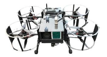
RAPTOR is the future of tactical counter drone systems. Completely autonomous - once launched by its operator it intercepts and defeats multi-rotor and fixed-wing drone threats with a munition or net then returns to its launch point for re-arming and re-use. Tiltrotor configuration permits precise attitude control for targeting accuracy with a coaxial quadcopter layout enabling racing drone performance.
